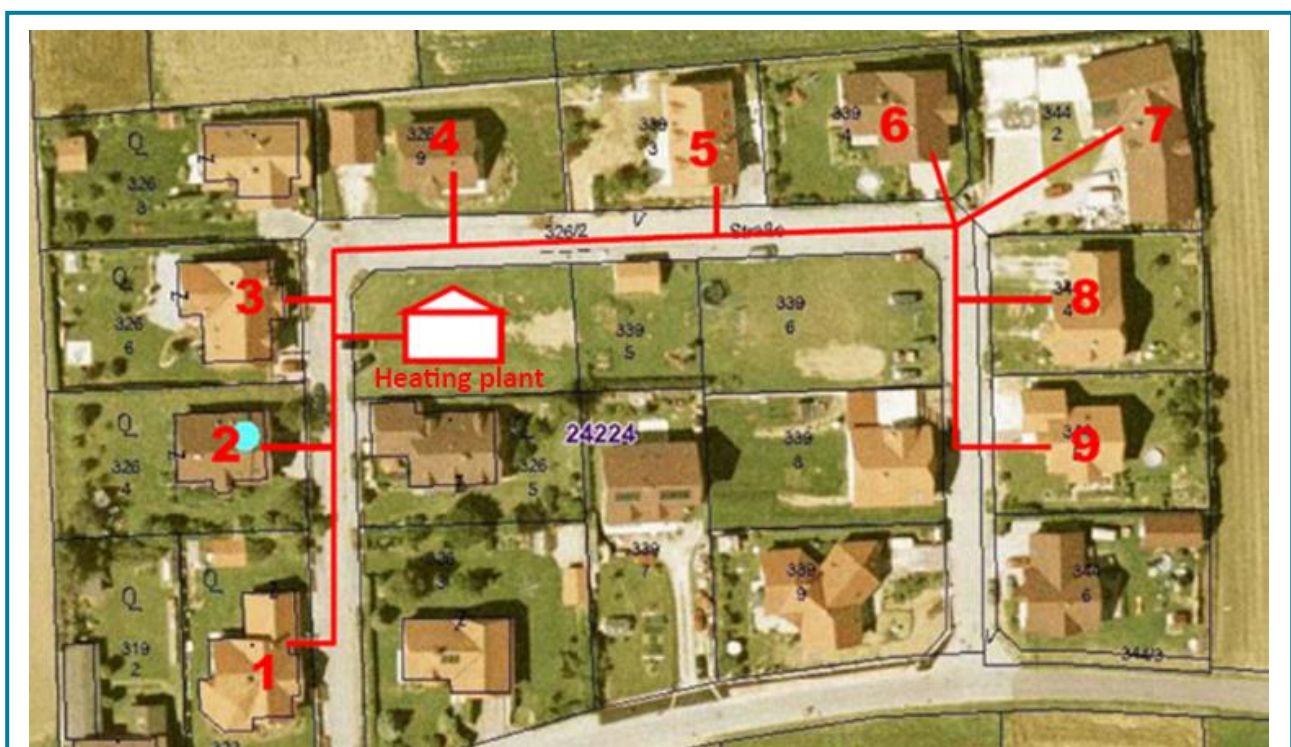
Figure 9 The use of wood-chip boilers in the residential sector to heat a group of houses
