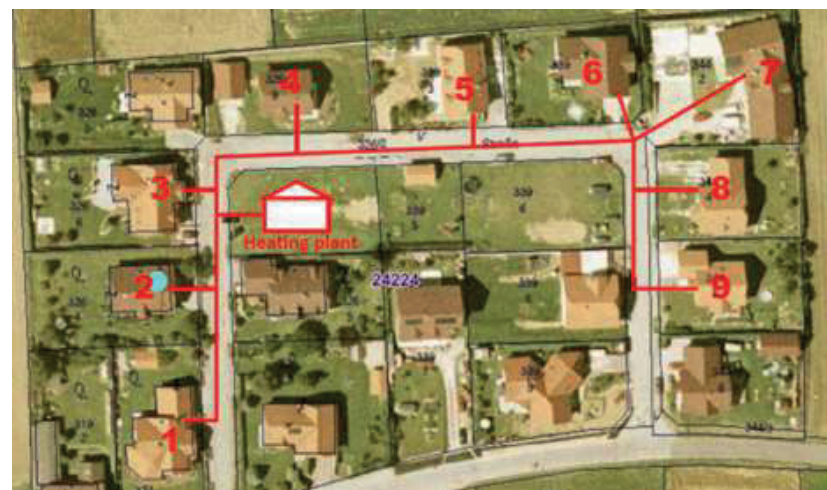
The use of wood-chip boilers in the residential sector to heat a group of houses
