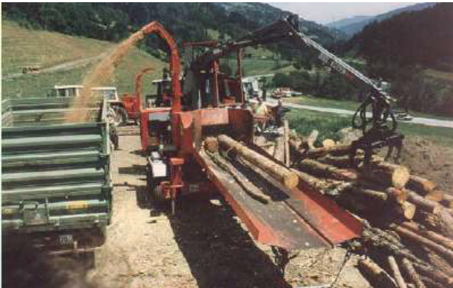
Wood chipper with mechanized feeding
